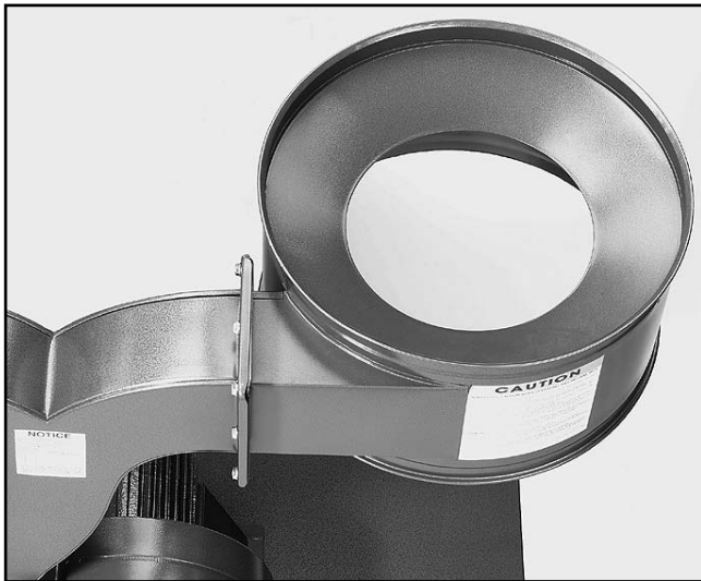
Figure 5. Attaching collector to outlet flange
